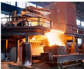
An old electric arc furnace pouring out steel into a small ladle car. The transformer vault can be seen at the right side. https://www.reuters.com
